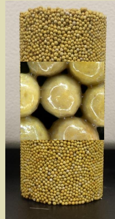
Proppant pack formed with zero closure stress
