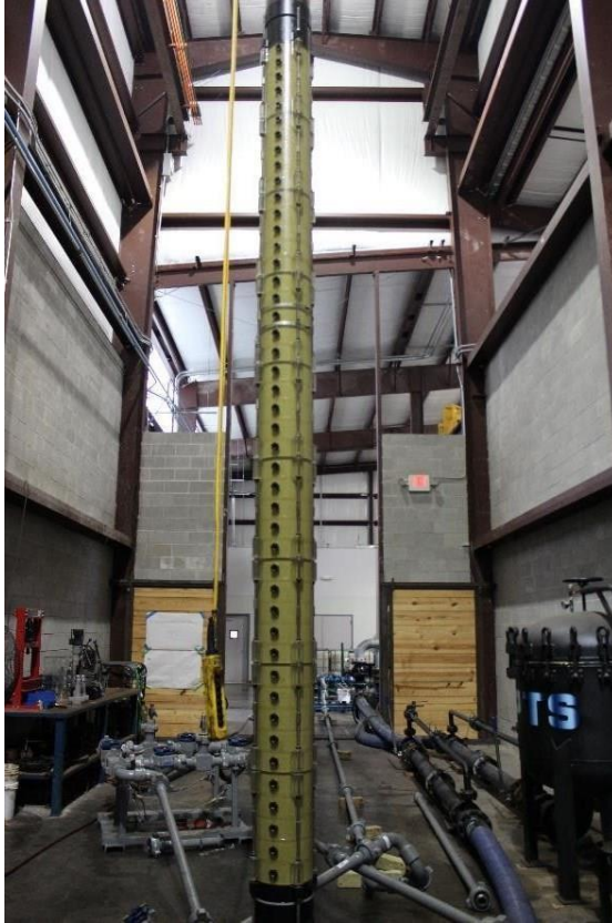
Fully Packed CHGP Assembly: Plexiglass Casing
