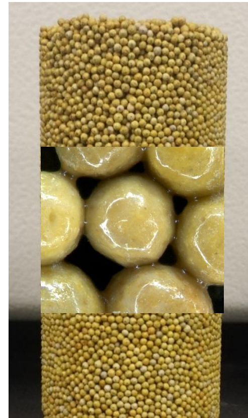
Proppant pack formed with zero closure stress @ 200F
