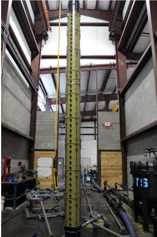
Fully Packed CHGP Assembly: Plexiglass Casing
