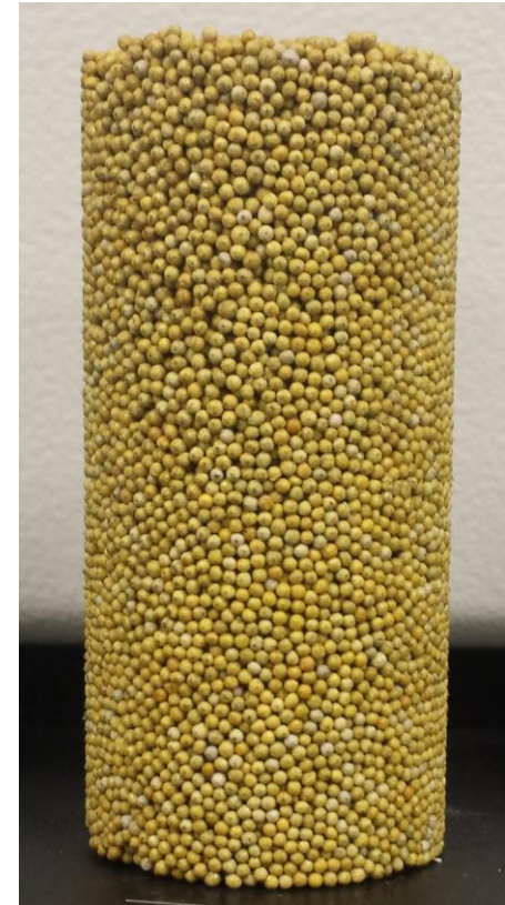
Proppant pack formed with zero closure stress
