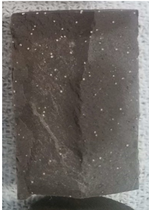
Cement Plug with fully suspended 40/70 CARBONRT
